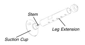
FIGURE 1 - ASSEMBLY OF THE LEG EXTENSIONS W/3-INCH SUCTION CUPS
